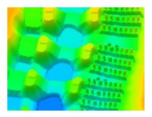
The proposed fish passage structure was modeled by Aquaveo using TUFLOW, a model well suited and very stable for analyzing 2D hydrodynamic effects that may result from the presence of hydraulic structures. A 0.25 meter modeling grid was used to represent the model domain which included several trapezoidal weirs, pools, two V-shaped channels, and large boulders.
