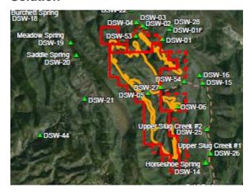
Aquaveo prepared recommendations for developing the conceptual flow and transport model. The conceptual model determines the appropriate model boundary conditions and to identify features that should be included in the numerical model. The model will address impacts such as seepage through the mine overburden fills and drawdown related to the pumping of a nearby water supply
