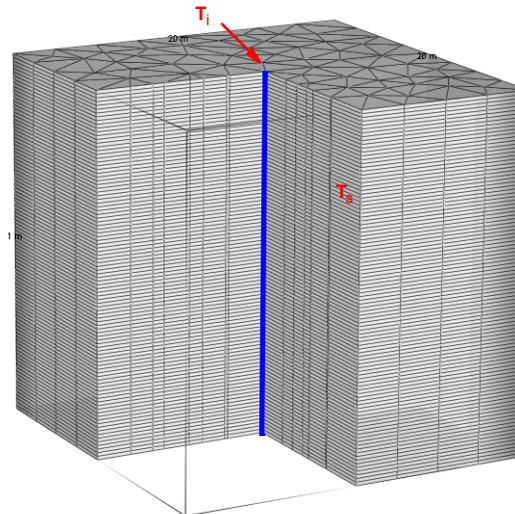
**Figure 1.16** Single BHE in a 3D mesh (exaggerated cut view).
