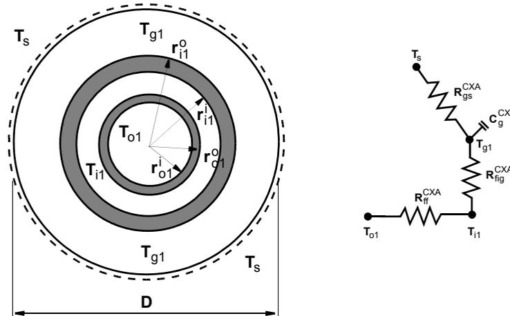
**Figure 1.4** Inner pipe-grout heat flux resistance relationships of a CXC borehole with annular inlet.
