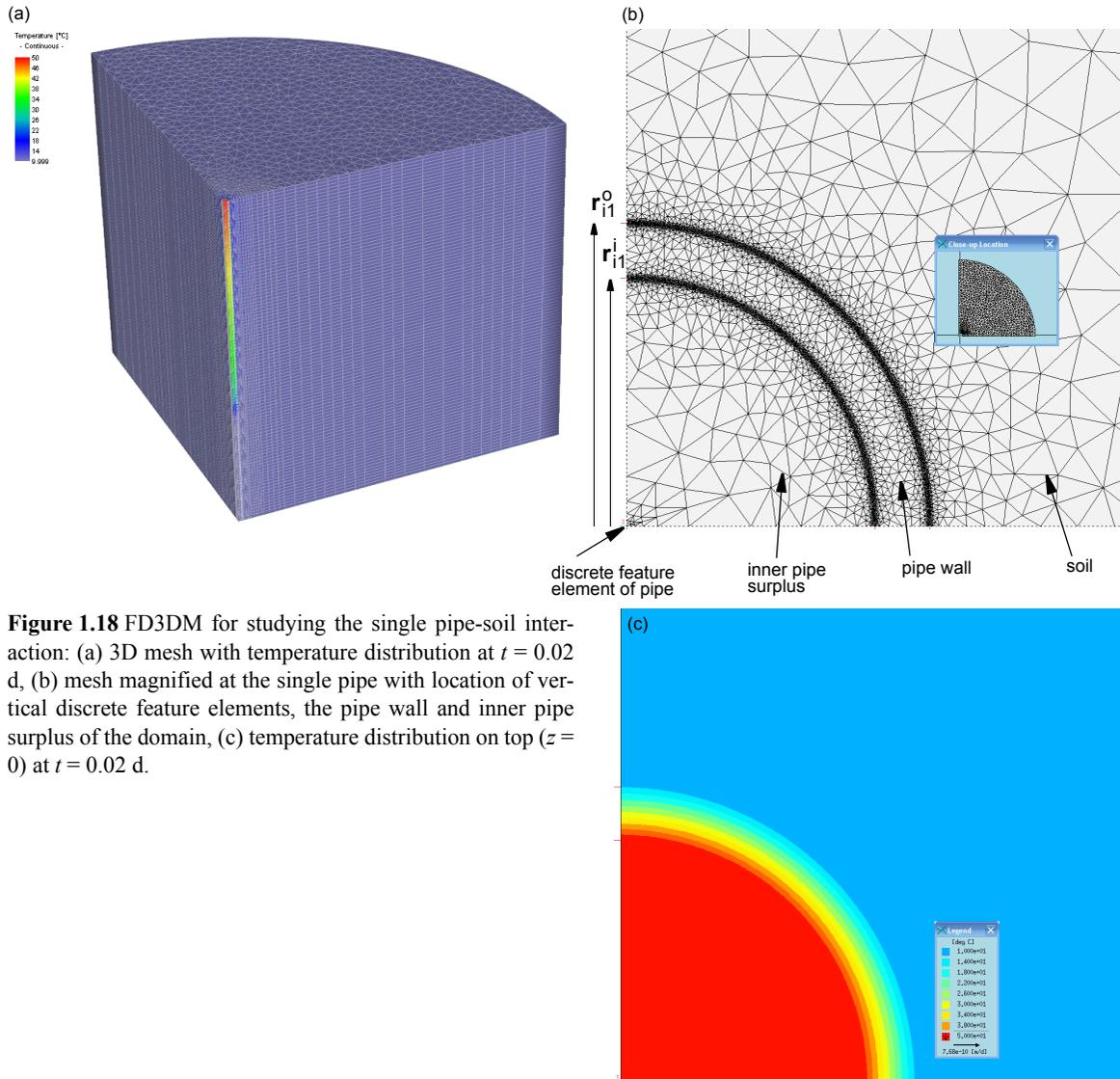
**Figure 1.18** FD3DM for studying the single pipe-soil interaction: (a) 3D mesh with temperature distribution at  $t = 0.02$  d, (b) mesh magnified at the single pipe with location of vertical discrete feature elements, the pipe wall and inner pipe surplus of the domain, (c) temperature distribution on top ( $z = 0$ ) at  $t = 0.02$  d.
