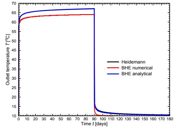
**Figure 1.23** Temperature history at pipe outlet of the CXA-type BHE for turbulent flow compared to Heidemann's solution.
