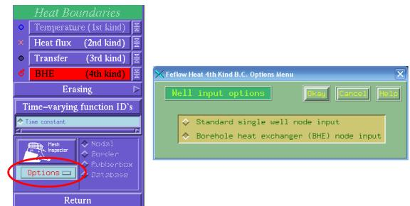
**Figure 1.8** Setting borehole heat exchanger node input via FEFLOW’s heat 4th kind BC option menu.
