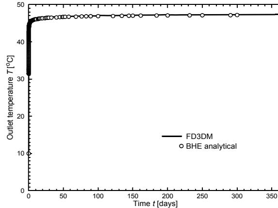
**Figure 1.30** Long-term outlet temperature history of the BHE solution in comparison to the fully discretized 3D model (FD3DM) solution measured at the pipe's outlet.
