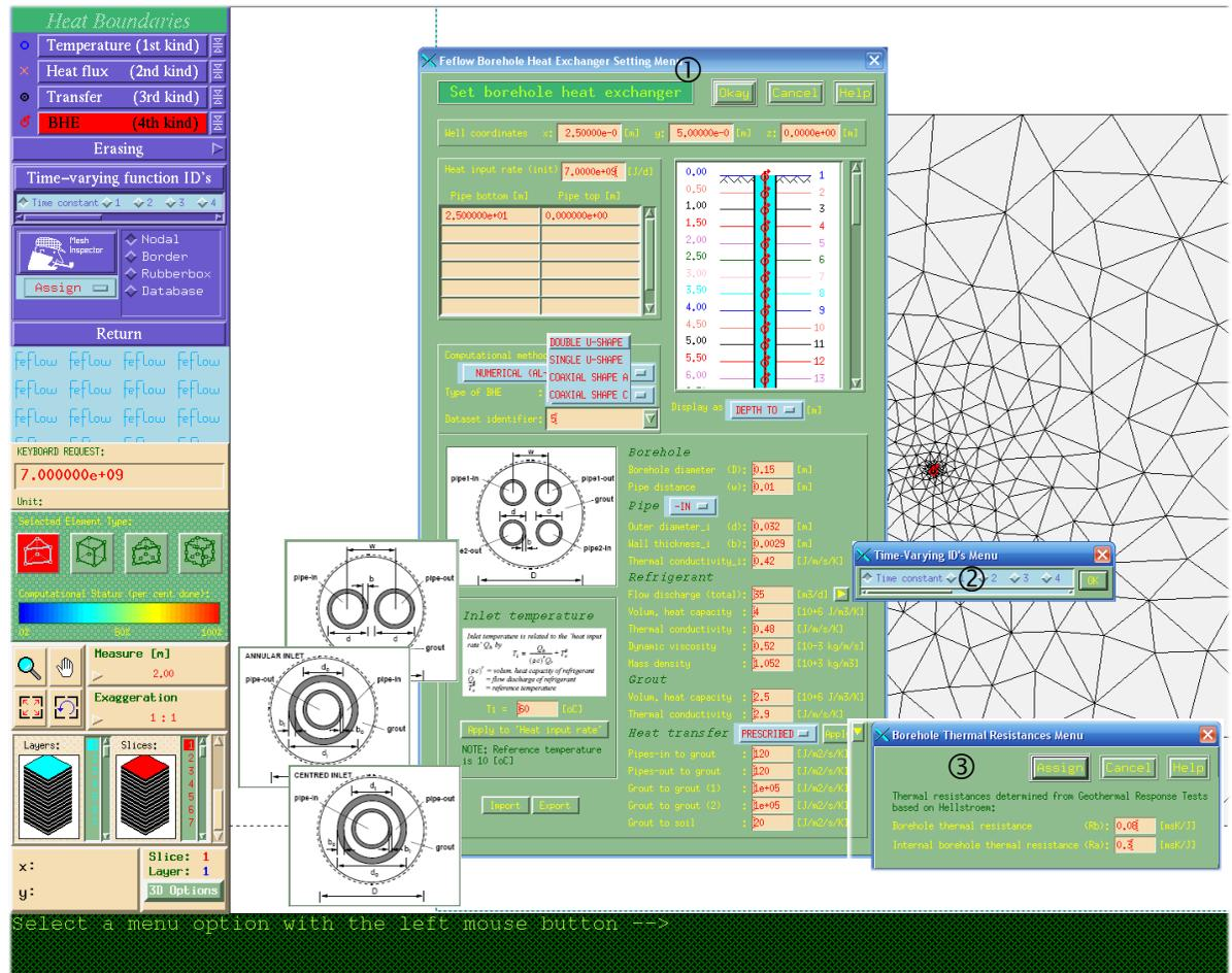
**Figure 1.9** FEFLOW's borehole heat exchanger setting menu: ① major BHE menu, ② optional input for time-dependent discharge  $Q_d(t)$  of refrigerant, and ③ optional input of thermal resistances  $R_b$  and  $R_i$  from thermal response tests.
