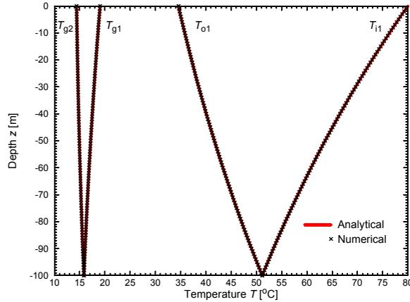
Figure 1.14 Analytical vs. numerical temperature distribution for 1U-type BHE.
