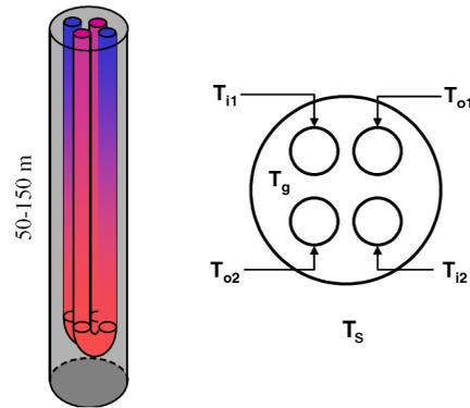
**Figure 1.1** Schematization of a 2U-type BHE (from Al-Khoury and Bonnier<sup>2</sup>).
