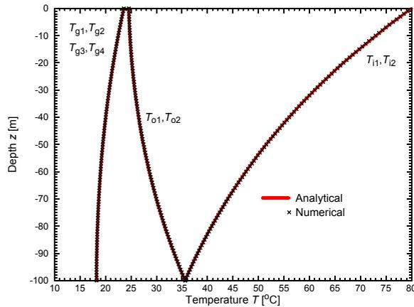
Figure 1.15 Analytical vs. numerical temperature distribution for 2U-type BHE.
