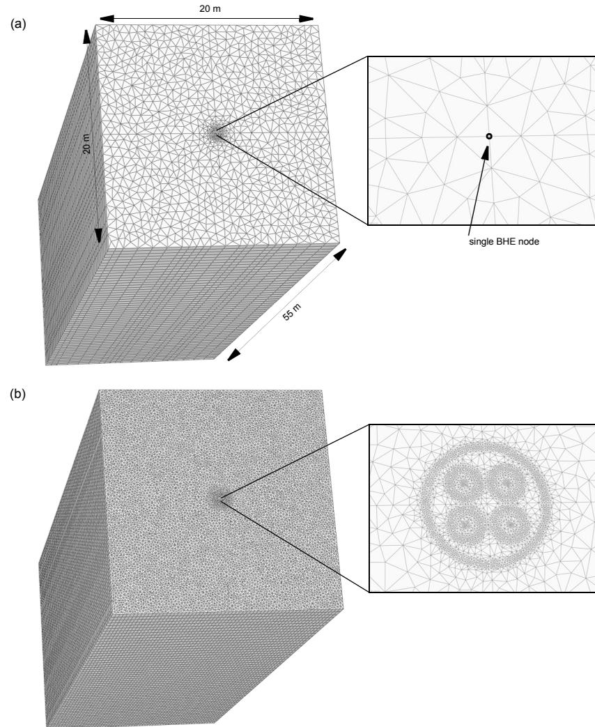
**Figure 1.28** Finite-element meshes for (a) BHE consisting of 130,185 pentahedral elements and (b) FD3DM consisting of 1,204,665 pentahedral elements. Both meshes are vertically discretized by 55 layers.
