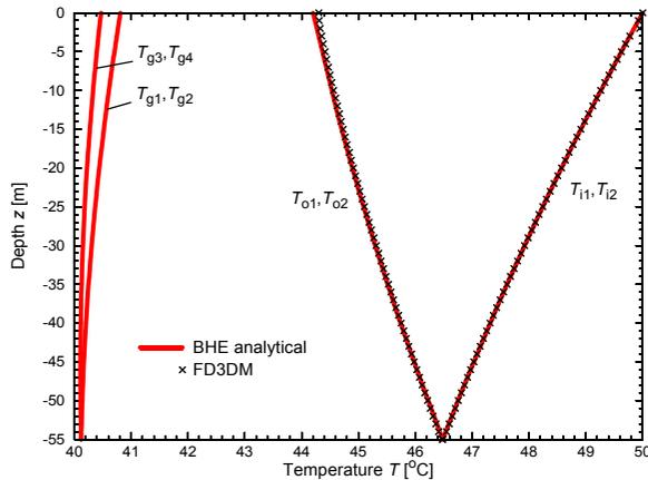
**Figure 1.31** Analytical BHE solution of temperature profile at  $t = 12$  hours in comparison to the fully discretized 3D model (FD3DM).
