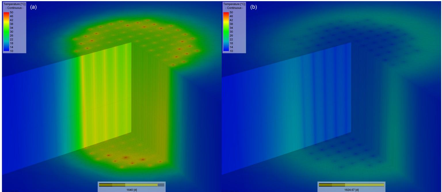
**Figure 1.34** Temperature distribution around the array of 80 BHE computed with FEFLOW and coupled with TRNSYS: (a) at the end of the heat injection period after 4 years and 180 days. (b) after 5 years.
