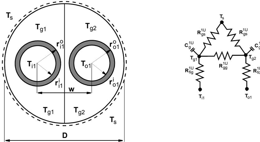
**Figure 1.3** Inner pipe-grout heat flux resistance relationships of a 1U borehole consisting of two pipe components and two grout zones.
