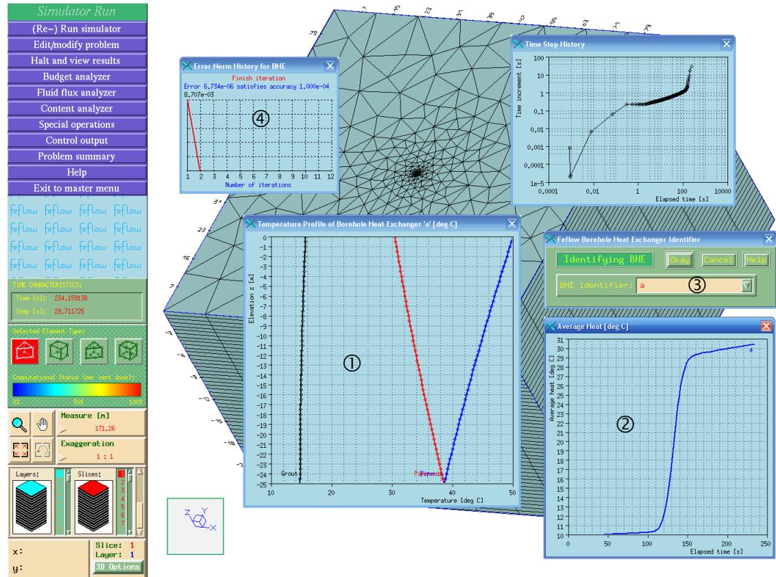
**Figure 1.10** BHE diagrams appearing in simulation: ① vertical temperature profiles, ② time history of pipe-top temperature on top  $T_{o1}(x_p, y_p, z_p, t)$ , ③ BHE's ID selector and ④ iteration history.
