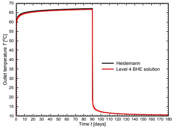
**Figure 1.27** Outlet temperature history of the CXA-type BHE for turbulent flow simulated with optimal mesh of refinement level 4,  $Y_4$  (analytical BHE solution) compared to Heidemann's solution.
