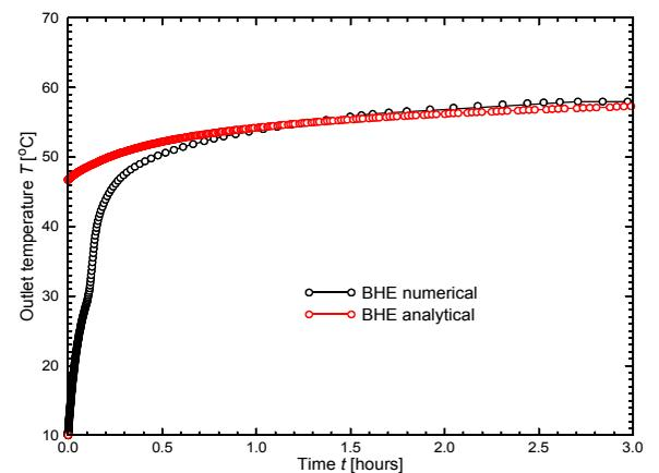
**Figure 1.24** Short-term temperature history at pipe outlet of the CXA-type BHE for turbulent flow.
