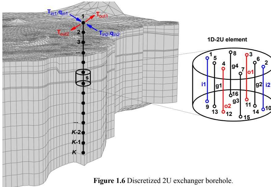
Figure 1.6 Discretized 2U exchanger borehole.
